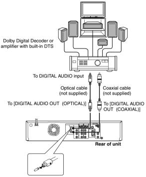
Note for connection: Remove the protection cap from the cable.
